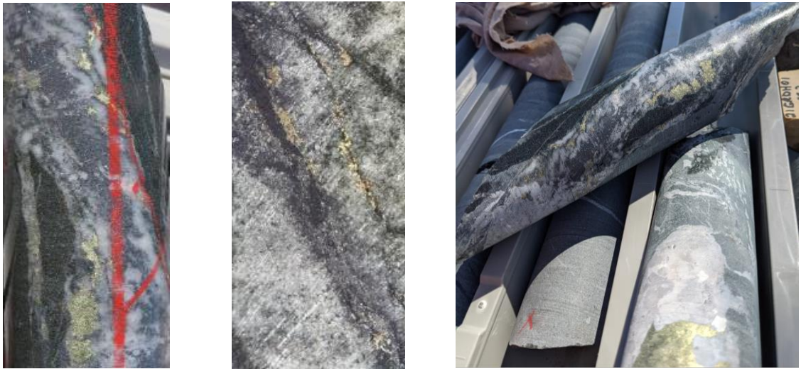
Figure 1: Osprey IOCG copper mineralisation (chalcopyrite) in drill core. 3
