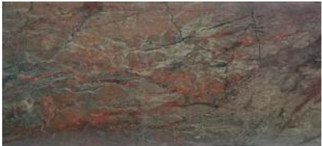
Figure 1: Osprey IOCG copper mineralisation (chalcopyrite) in drill core. 3
