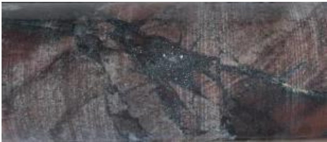
Figure 2: Alteration and veining in Osprey drill core indicative of IOCG signatures 3 .
