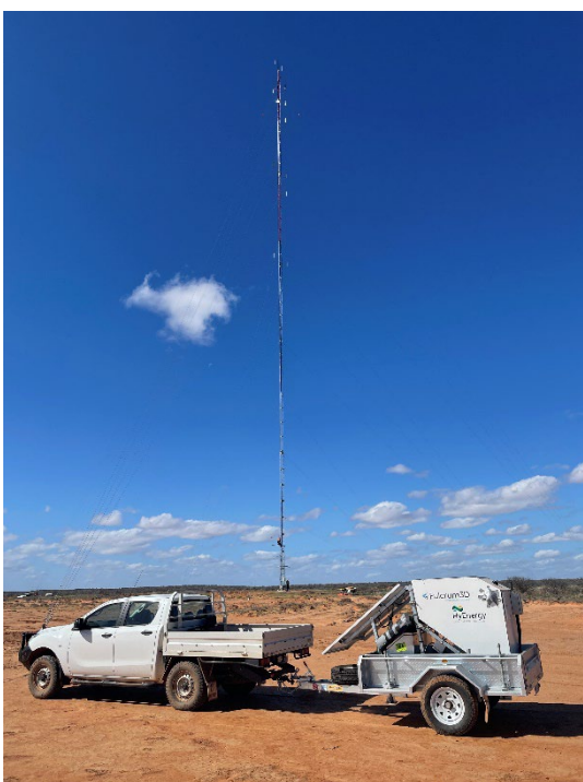
Met-Mast and SODAR on the HyEnergy™ Project Licence area
