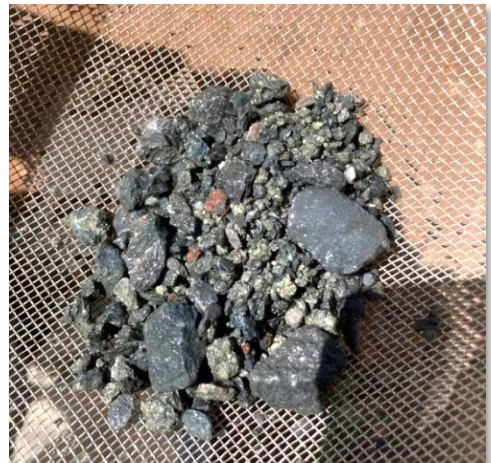
Plate 1: RC drill chips from hole 22MERC016 sample (88 to 89m) showing strong chalcopyrite
