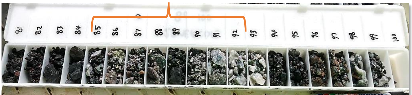
Plate 2: Chip tray from hole 22MERC016 (80m to 100m) showing sulphide mineralisation
