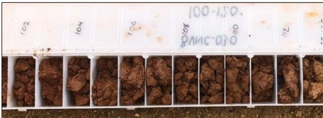
Figure 2. Deeply weathered saprolite/clay and Ni-Cu-PGE zone from 101m in BVNC030. (12m @ 0.51% Ni, 605ppm Cu, 236ppb PGE from 101m)
