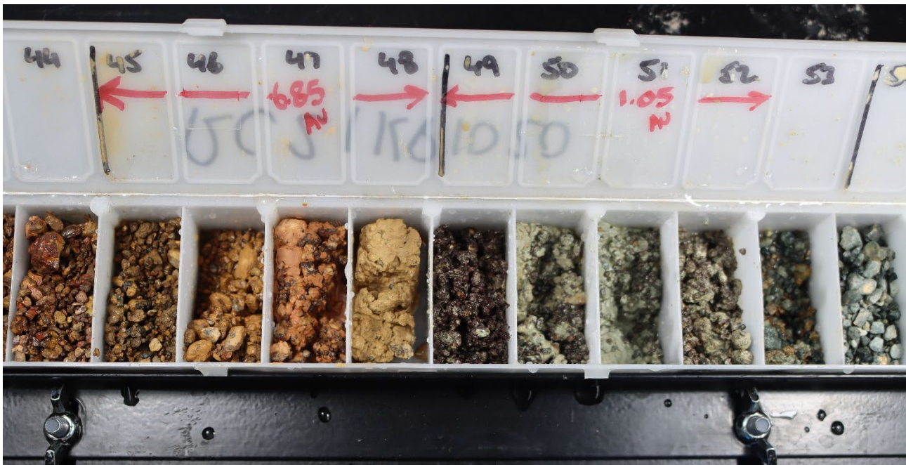
Figure 5: Oxidised quartz-gravel and clays within RC21KP1020 situated at the contact with saprock. Composite grades are written on chip trays. 1m re-splits of samples recorded 2m @ 7.89 g/t Au, 0.19 % Cu, 0.35 g/t Ag from 44m including 1m @ 14.4 g/t Au from 44m.
