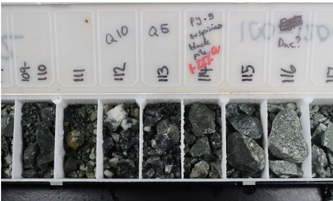
Figure 6: RC21KP1012 with 1m @ 0.52 g/t Au, 1.22 % Cu and 7.99 g/t Ag from 113m. Mineralisation is associated with sulphides and is situated within the bedrock and is interpreted to be the Gift Structure and not related to a paleochannel setting.
