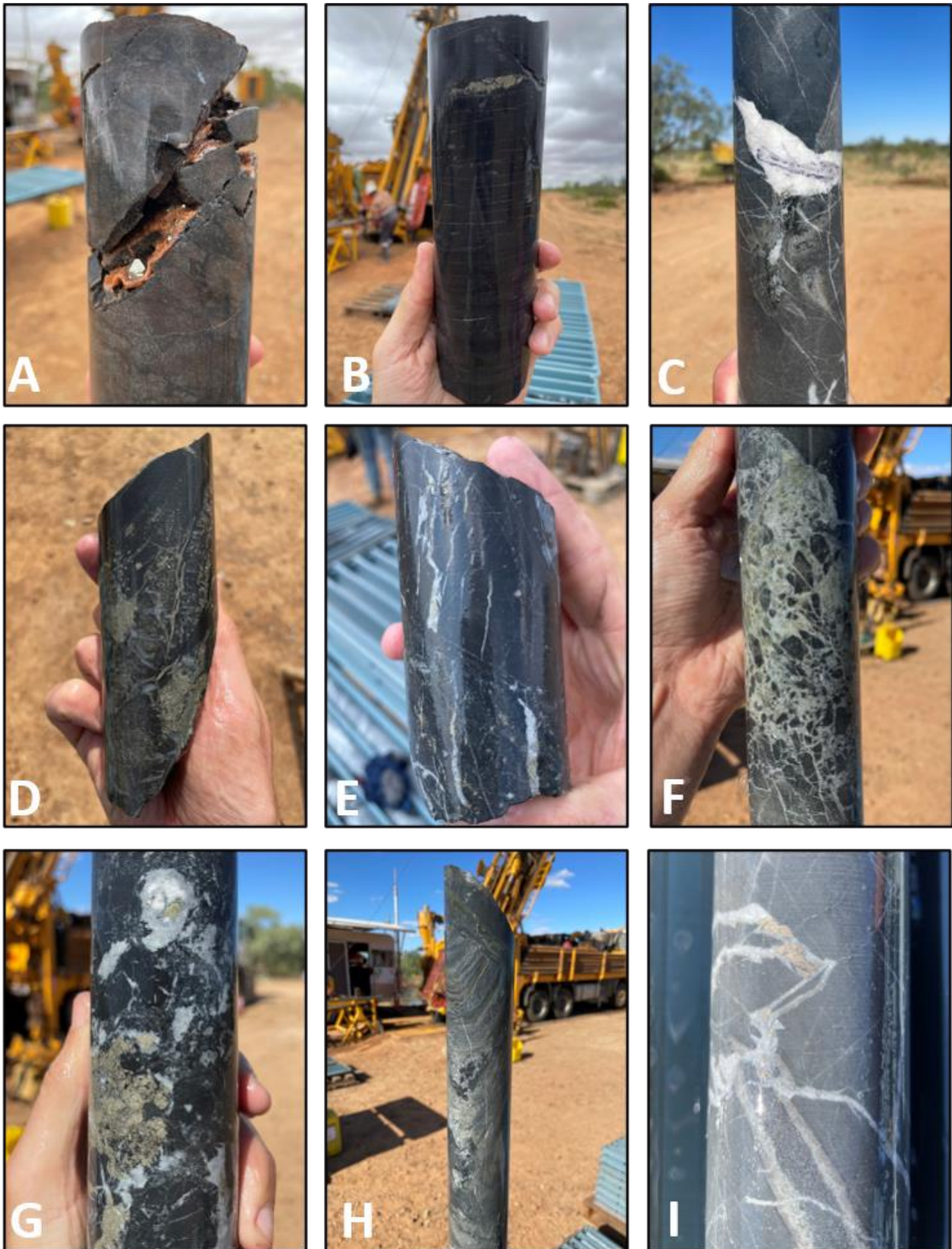
Figure Ap2(a): FW220006 core photo collage showing the progression of geology, alteration and veins down the hole, including: A) coarse-grained, euhedral pyrite with carbonate in siltstone at 262m, B) shale with laminated and disseminated pyrite at 294m, C) quartz-calcite-fluorite-pyrite veining at 313m, D) pyrite-quartz veining in graphitic schist at 632m, E) fault offset quartz-pyrite veinlets in black shale at 648m, F) quartz-carbonate-dolomite breccia zone within metasiltstone at 679m, G) chalcopyrite-carbonate and quartz-pyrite-carbonate veining in graphitic schist at 685m, H) faulted and brecciated shale-siltstone with carbonate laminations and dolomitic overprint at 708m, and I) pyrrhotite-chalcopyrite-quartz-carbonate veining in dolomitised metasiltstone at 723m.
