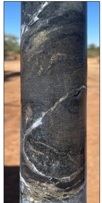
Figure 1: Semi-massive pyrrhotite-pyrite-(chalcopyrite) intersected at 866m over a downhole interval of 25cm in FW220006.
