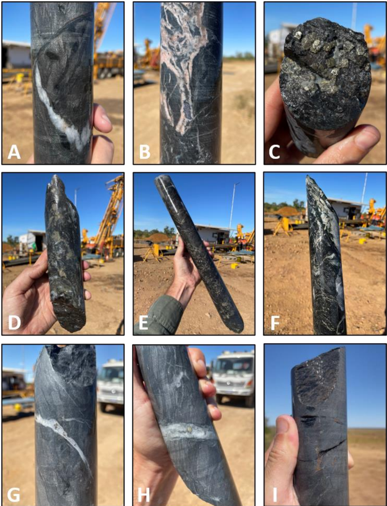
Figure Ap1(b): FW220002 core photo collage showing the progression of geology, alteration and veins down the hole, including: A) quartz vein truncated by a younger quartz-chlorite-haematite veinlet at 603m, B) chalcopyrite and galena in quartz-carbonate veining at 653m, C) coarse-grained, euhedral pyrite cubes at 655m, D) quartz-pyrite veining in graphitic schist at 657m, E) pervasive pyrrhotite veining and laminations in graphitic schist at 660m, F) quartz-pyrite-(chalcopyrite) veining in graphitic schist at 662m, G) quartz veins with rare sphalerite and chalcopyrite at 664m, H) rare chalcopyrite in quartz-chlorite vein at 667m, and I) sphalerite disseminated in shale at 669m.
