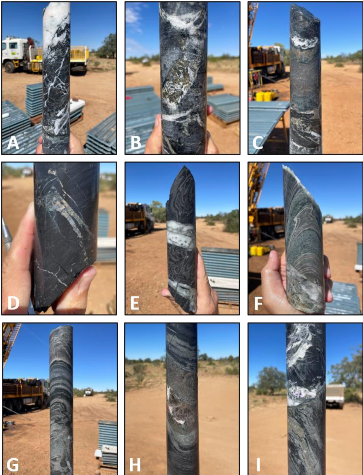
Figure Ap2(b): FW220006 core photo collage showing the progression of geology, alteration and veins down the hole, including: A) quartz-pyrite-carbonate veining and brecciation in shale-siltstone at 780m, B) coarse-grained biotite in quartz-carbonate veins at 856m, C) semi-massive pyrrhotite-pyrite-(chalcopyrite) in quartz-carbonate veined and dolomitised shale-siltstone at 866m, D) quartz-pyrrhotite-chalcopyrite veins in shale at 881m, E) quartz-carbonate veins in folded black shale at 886m, F) dolomitised siltstone cut by quartz-carbonate-pyrite veins at 895m, G) dolomitised siltstone with quartz-carbonate-pyrite veins at 898m, H) dolomitised siltstone with quartz-carbonate-fluorite (?) veining at 941m, and I) quartz-carbonate-pyrite-fluorite veining in dolomitised siltstone at 960m
