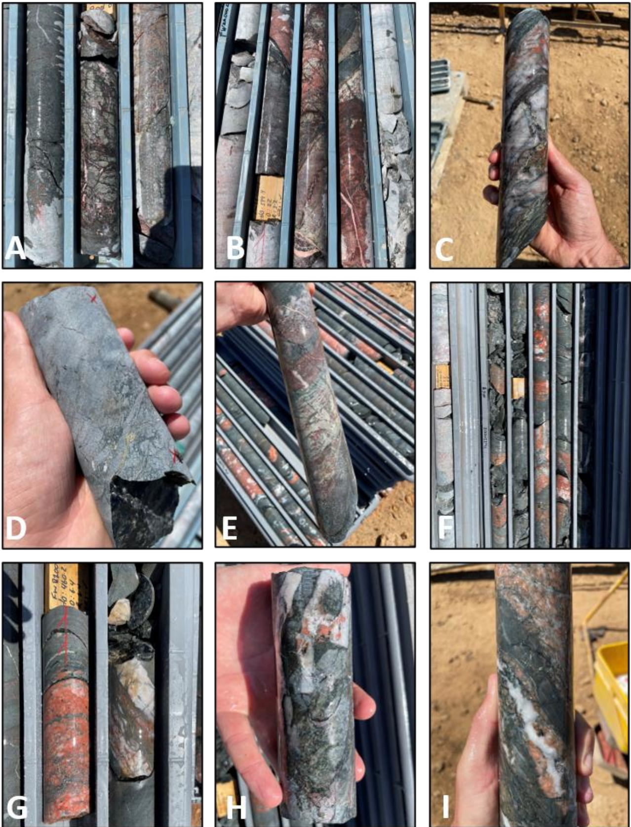
Figure Ap1(a): FW220002 core photo collage showing the progression of geology, alteration and veins down the hole, including: A) chlorite-haematite-quartz-carbonate breccia zone at 396m, B) haematite-quartz-chlorite-carbonate veining and brecciation at 400m, C) quartz-haematite-kspars-chlorite vein at 410m, D) chalcopyrite in metasilstone at 425m, E) quartz-epidote-chlorite-haematite-pyrite veining at 445m, F) quartz-haematite-kspars veining at 450m, G) haematite stained quartzite with muscovite (left) and quartz-haematite veining (right) at 460m, H) quartz-chlorite-haematite-kspars veining at 495m, and I) quartz-pyrite veining in quartzite-metasilstone at 577m.
