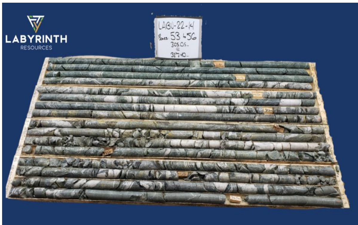
Figure 1 - Core tray containing visually interpreted Boucher intercept from 310m - 326m in LABU-22-14
