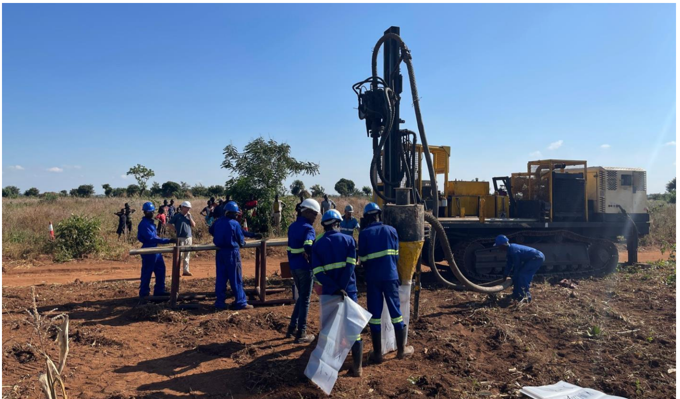
Figure 1: Air-core rig drilling its first hole at Kasiya observed by MRE Competent Person Mr Richard Stockwell of Placer Consulting.
