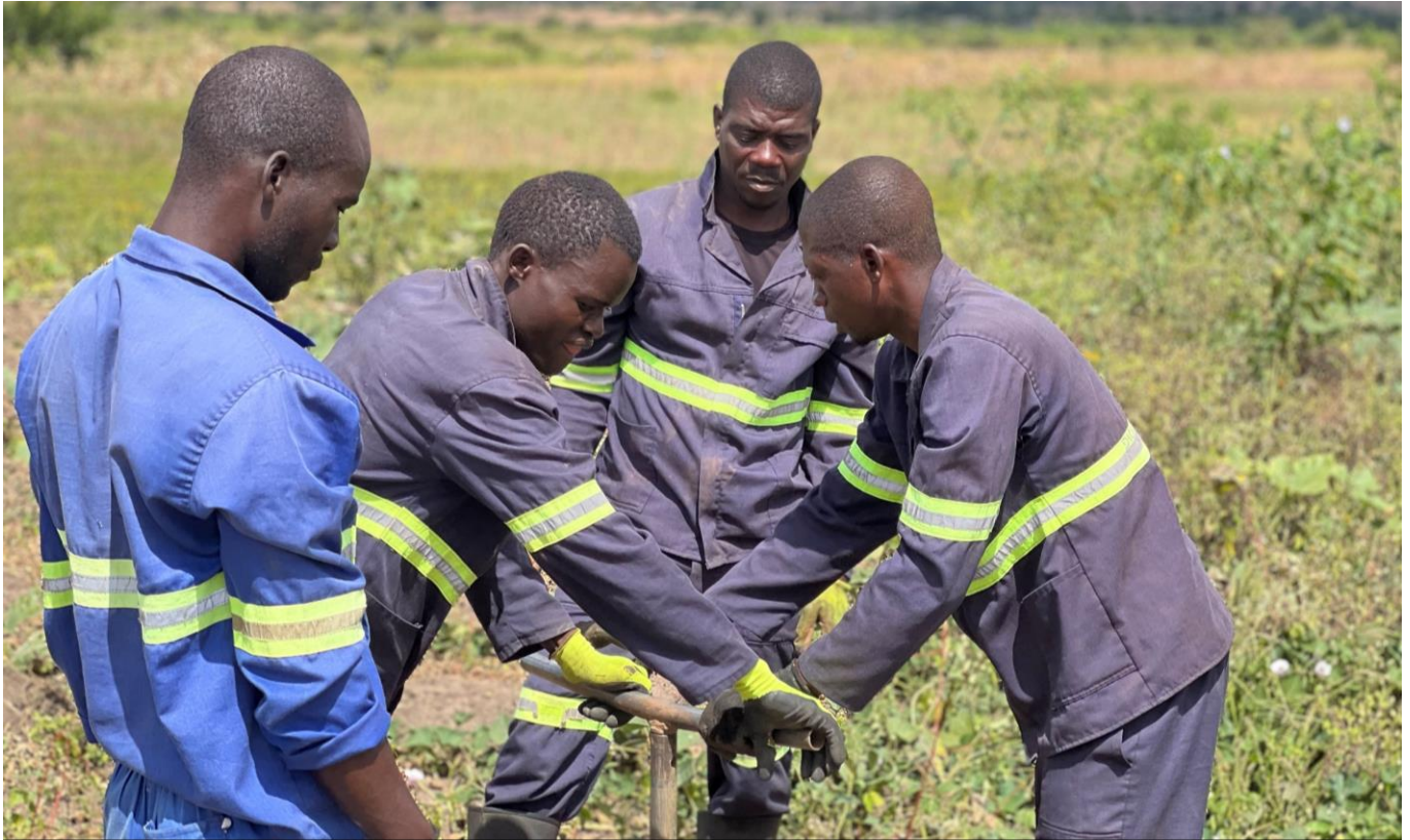
Figure 4: Hand-auger team drilling a regional reconnaissance hole.
