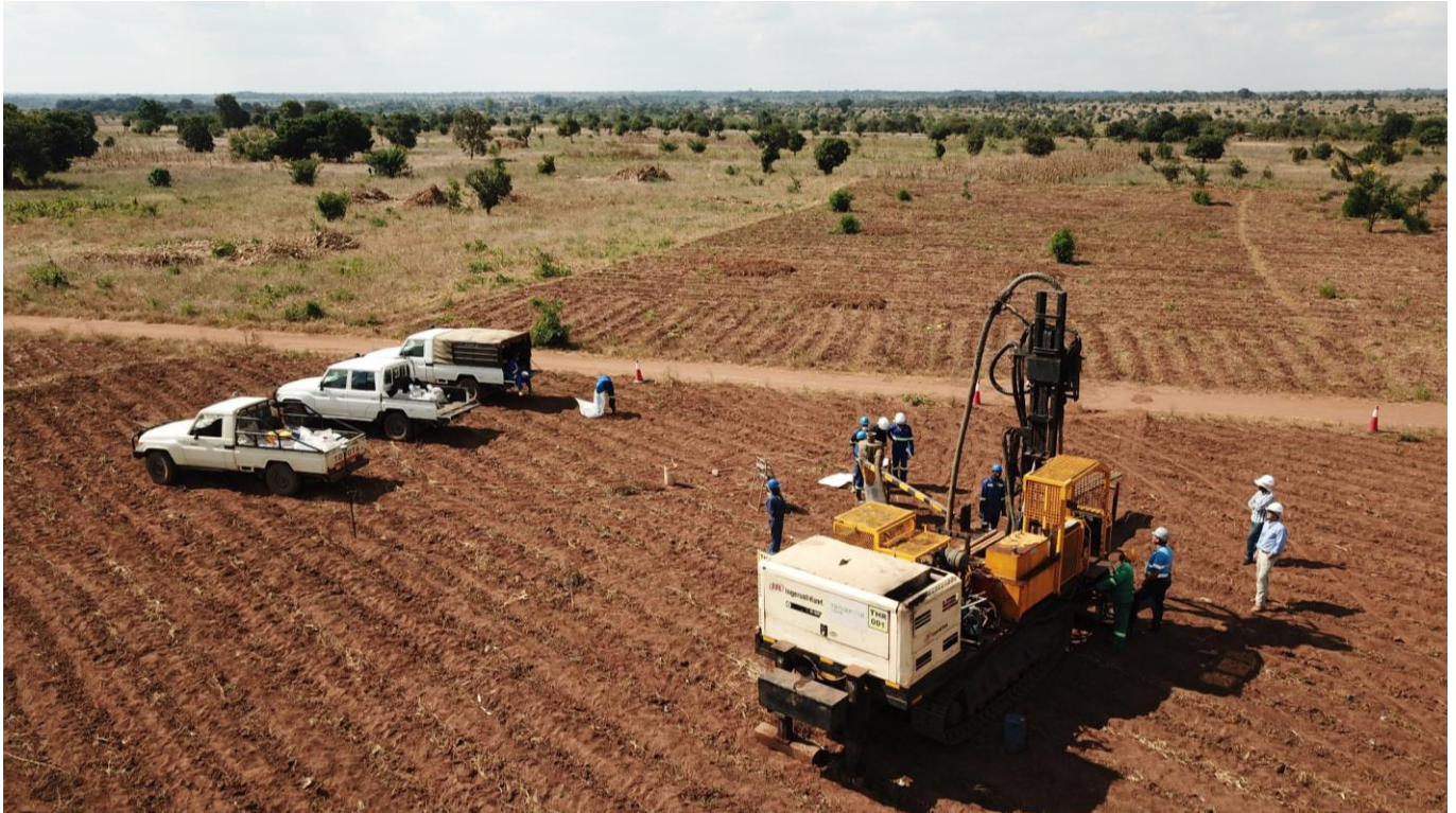
Figure 3: Drone photo of air-core drilling at Kasiya overseen by Sovereign's geology team.
