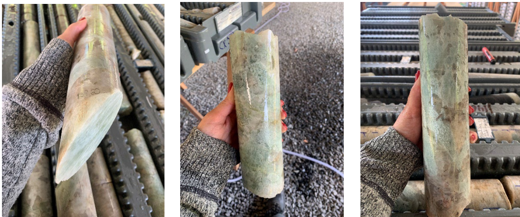
Figure 3: Drill core from SADD017 showing large light-green fresh spodumene crystals
