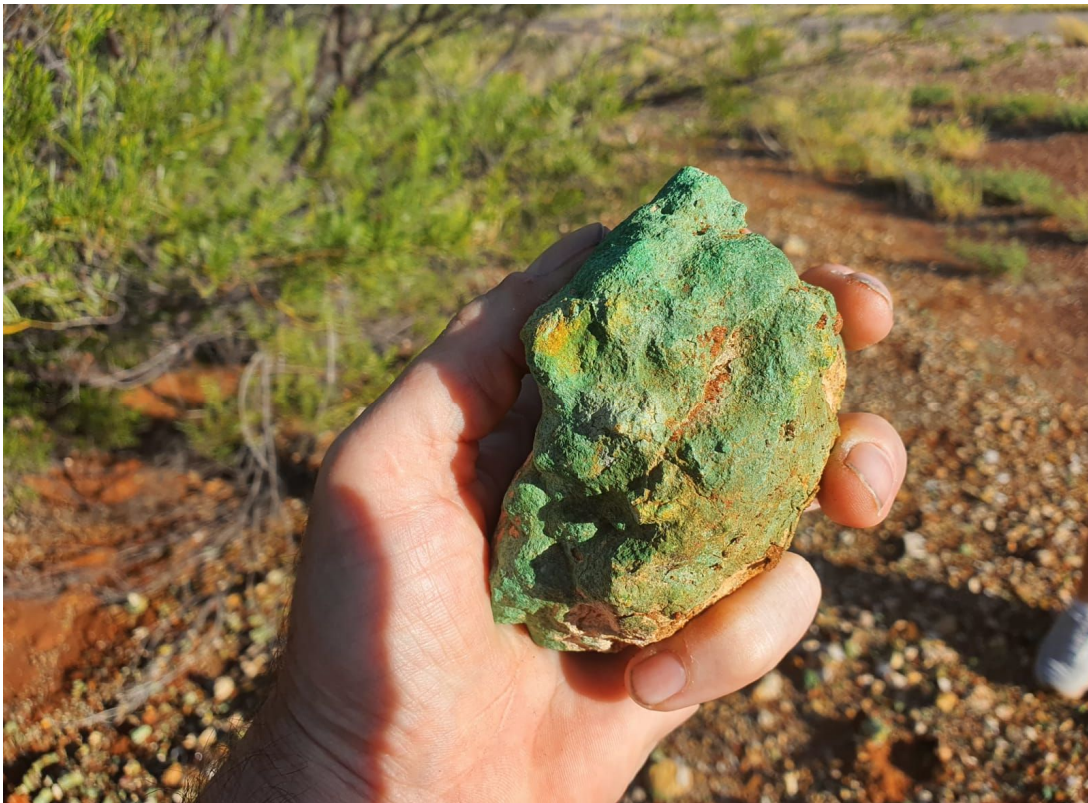
Figure 2 Crosswinds Copper Gold Project - Malachite (copper carbonate) mineralisation exposed in table drain
