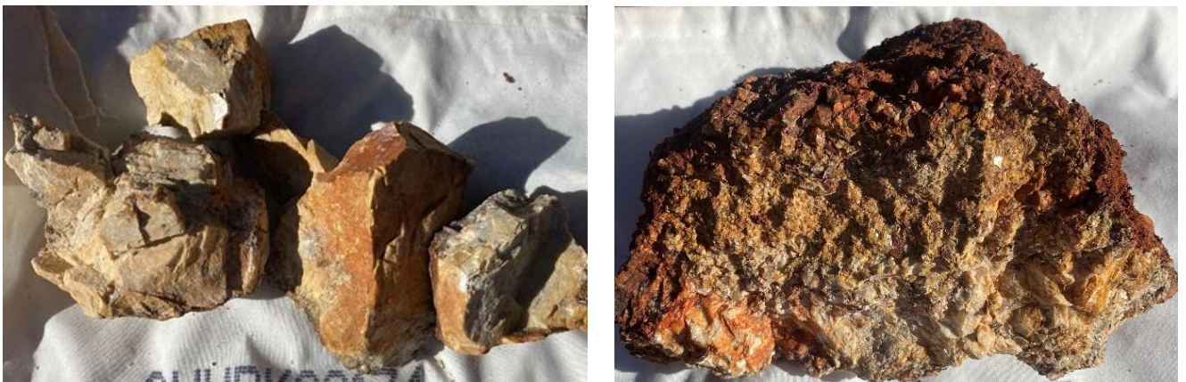
Figure 3 - Rock chip samples: (A). Blocky K-Feldspar; lithium (10ppm Li), beryllium (13ppm Be), caesium (49ppm Cs), niobium (28ppm Nb), tantalum (43ppm Ta) and rubidium (2,020ppm Rb); (B) Weathered pegmatite containing feldspar, mica, and quartz; lithium (168ppm Li), beryllium (19ppm Be), caesium (67ppm Cs), niobium (53ppm Nb), tantalum (22ppm Ta) and rubidium (1,015ppm Rb).
