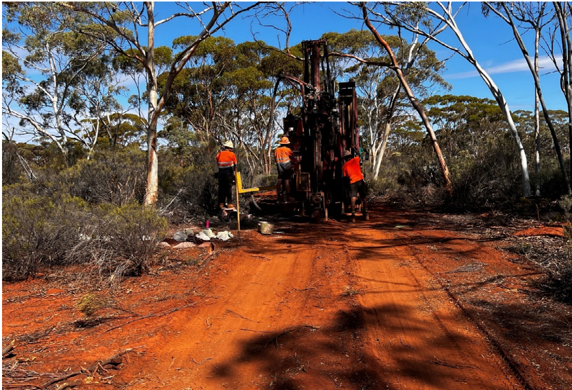
Image 3 – Air core drill rig on a regional exploration line.
