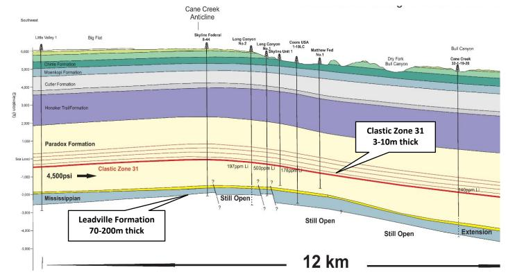
Schematic Cross Section through the Paradox Basin Project
