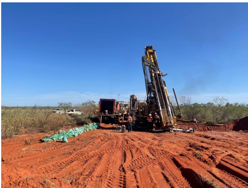
Image 1 RC drilling at the Highway Ni-Co-Cu-Pd deposit.
