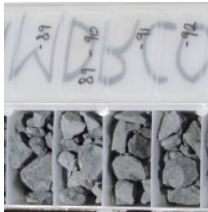
Image 4 / RC drill chips: 21MDRC033 88-92m (4m @ 1.27 % Cu & 212 ppm Co sulphide chalcopyrite and chalcocite mineralisation)
