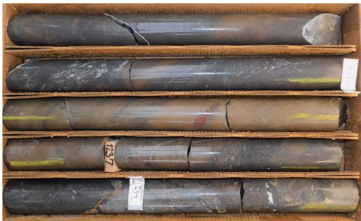
Figure 1: Photo of massive and semi-massive sphalerite (zinc sulphide – brown) and magnetite in drill hole WD22-03. This interval contains 47.59% Zn, 435.88g/t In from 376.26 – 377.02m (1234.5 - 1237ft) downhole.
