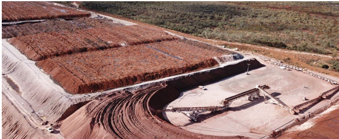
Ore Being Stacked on Heap Leach Pads, June 2022.
