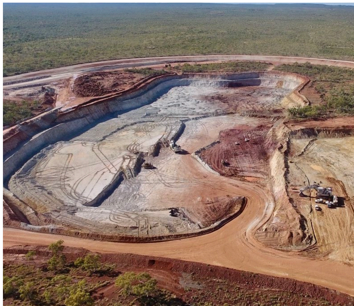
Mining at east pit. Ore can be seen on RHS of pit as darker coloured material.
