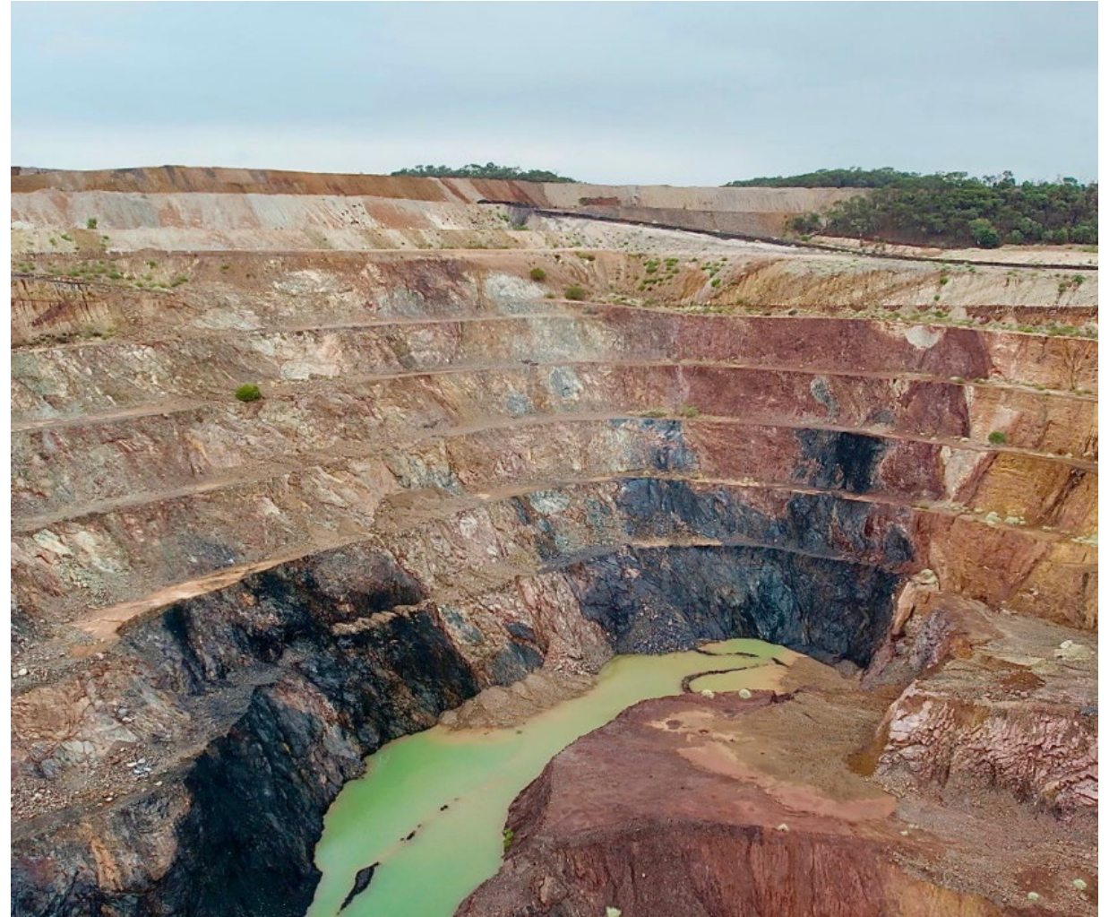
Flying horse pit showing progression from oxide at top of pit to transition then fresh or sulphide material at the bottom of pit
