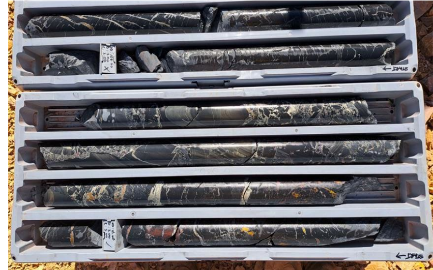
Diamond drill core of sulphide copper mineralisation from drillhole MTKD010 at Flying Horse pit.
