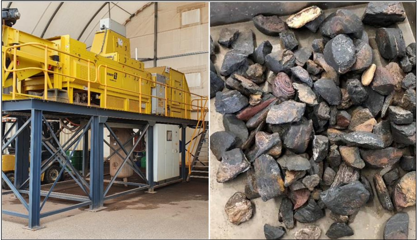
Figure 2. The Steinert ore sorter at Bibra Lake, Perth that was used to test +18mm samples from Flanagan Bore. The right-hand image is the +18mm material from the LR01 Lower composite
