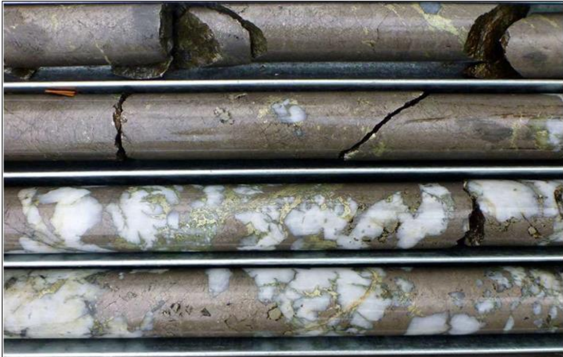
Figure 15: Massive Sulphides and Quartz Breccia in TALRCDD003 from 156m to 161m
