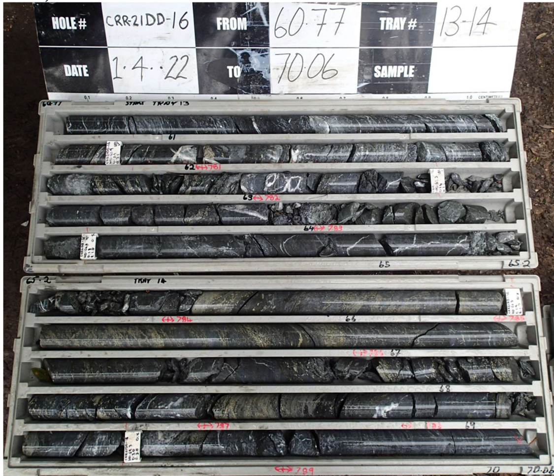
Figure 1: CRR21DD_16, interval comprising samples 42781-42788 assaying 7.6m @ 5.9% Zn, 1.16% Pb, 0.19% Cu, 7.23g/t Ag, 0.03g/t Au from 62-69.6m downhole including 1.3m @ 13.47% Zn from 65.60-66.90m (NQ core, 50mm diameter)
