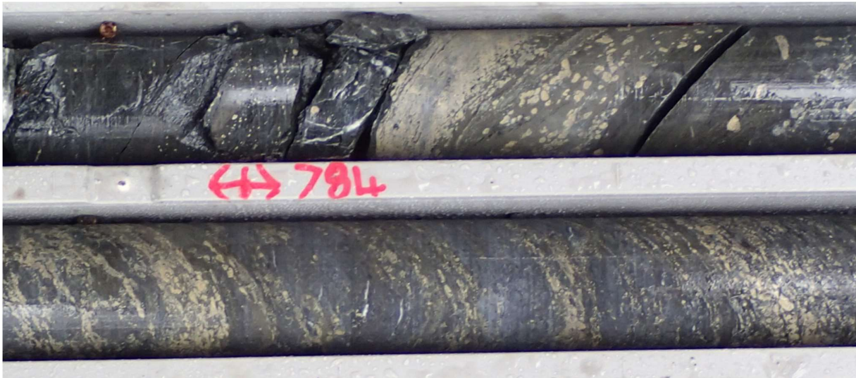
Figure 3: CRR21DD_16, interval comprising samples 42855-42857 assaying 3.1m @ 9.21% Zn, 4.66% Pb, 1.97% Cu, 59.67/t Ag, 0.33g/t Au from 163.2-166.3m downhole from 163.2-166.3m downhole (NQ core, 50mm diameter)
