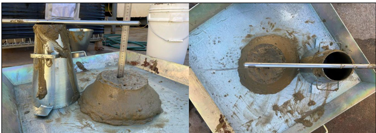
Figure 6: Slump Test (200mm) picture of 4% GP cement
