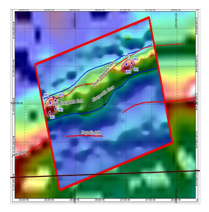
Figure 2: Chargeability image and interpretation from GAIP grid over magnetic image illustrating the location of the RC holes drilled.
