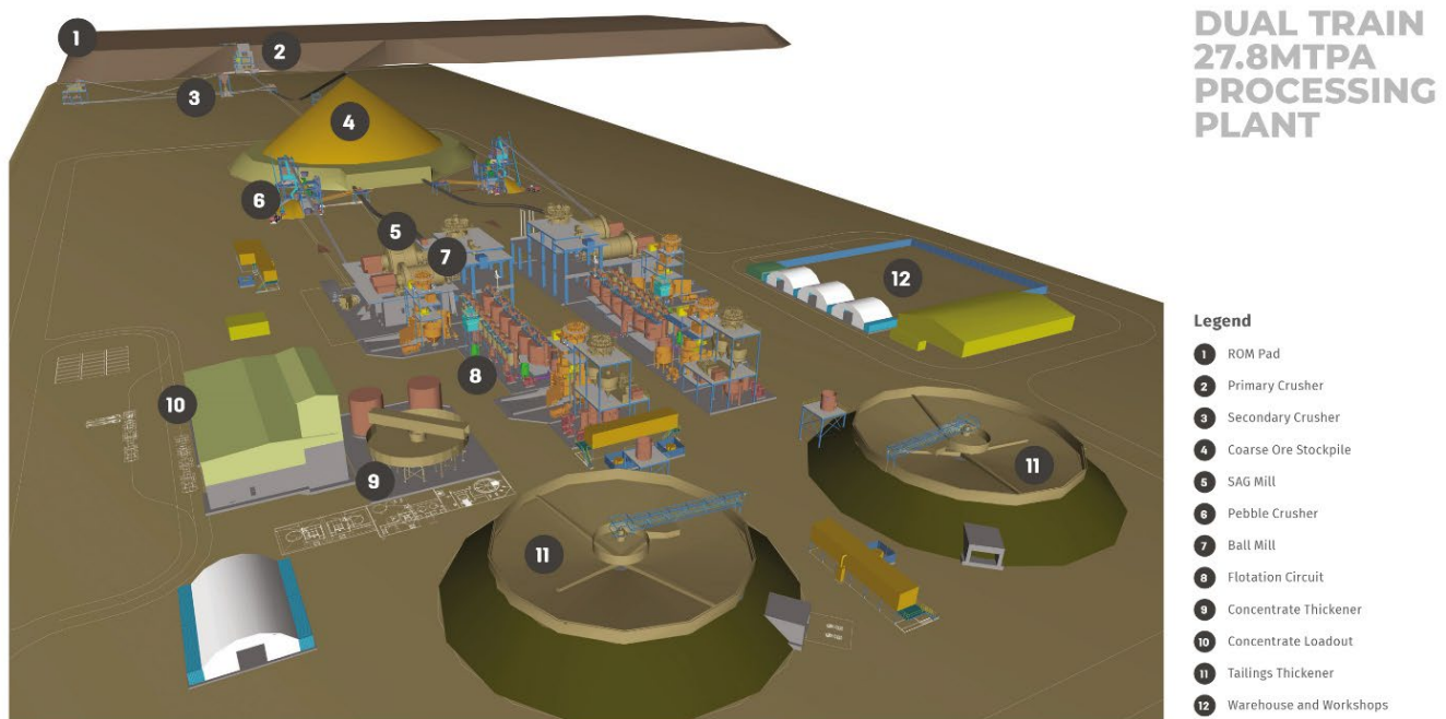
Figure 1: Preliminary layout for the process plant showing a crushing circuit (2,3) and coarse ore stockpile (4) feeding dual grinding mills (5,6&7) and flotation circuits (8). The dual train design was to allow staged developments and reduce up front capital costs. The option now being evaluated is based on a single ~27Mtpa plant through the use of larger equipment. The single train is expected to deliver significant savings in capital and operating costs, which are likely to outweigh the benefit of a staged development.
