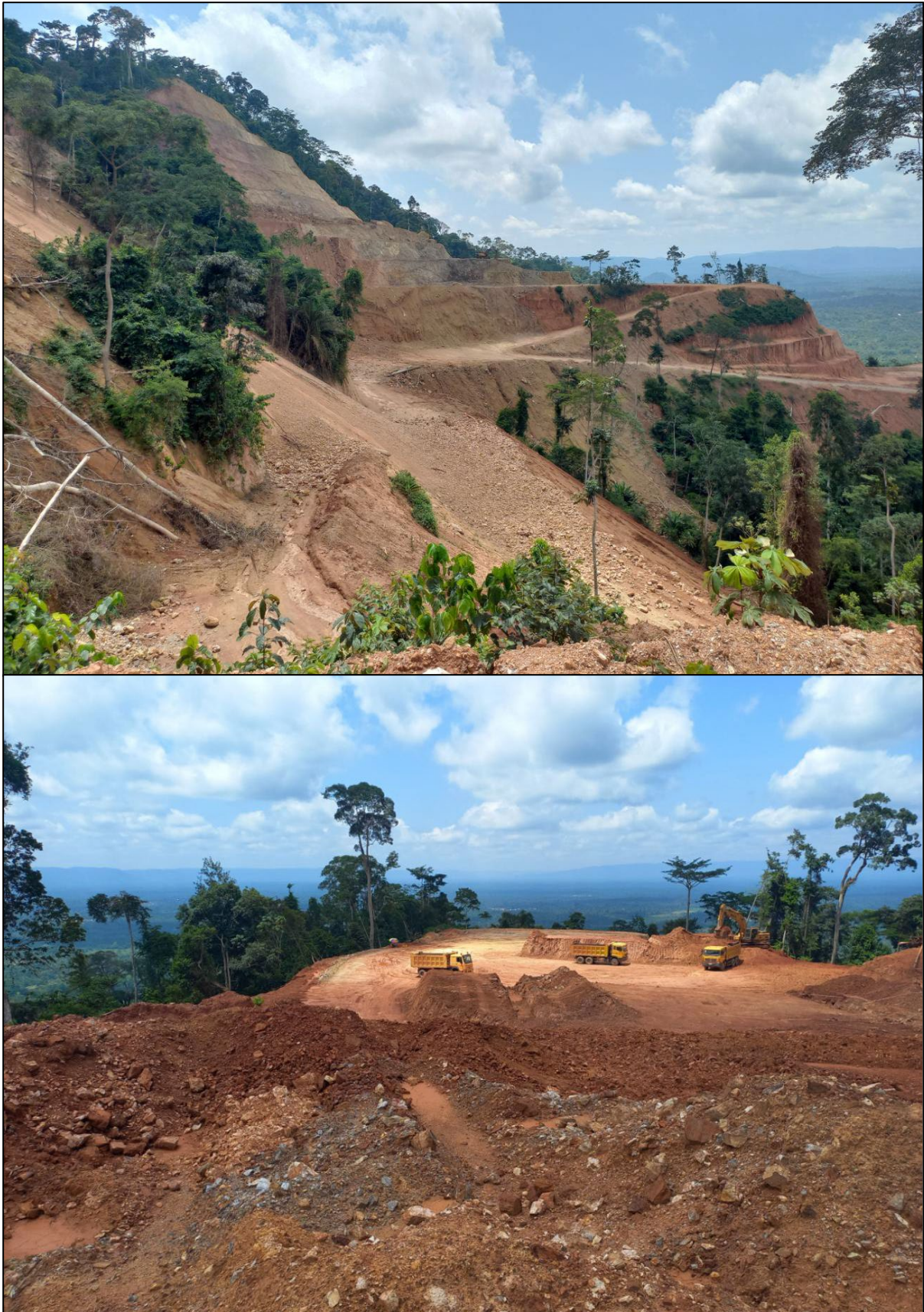
Figure 1; Photos showing mining activity at the Akoase Project in Ghana. Top: View to the NE of 5m benches in the Northern end of the Akoase Project. Bottom: Active mining taking place at the Akoase Project at the time of the site visit.
