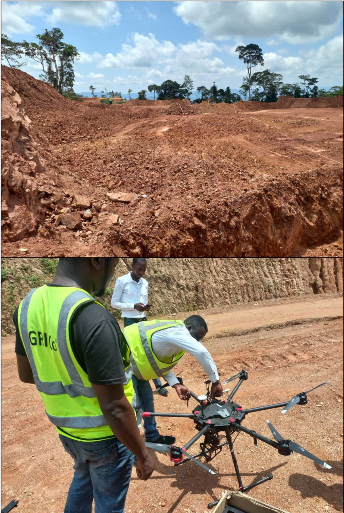
Figure 2; Top: Photo of mining bench with ore blocks demarcated with white tape; Bottom: SRK contracted surveyors setting up a drone for topographical survey to determine extents of mining activity.
