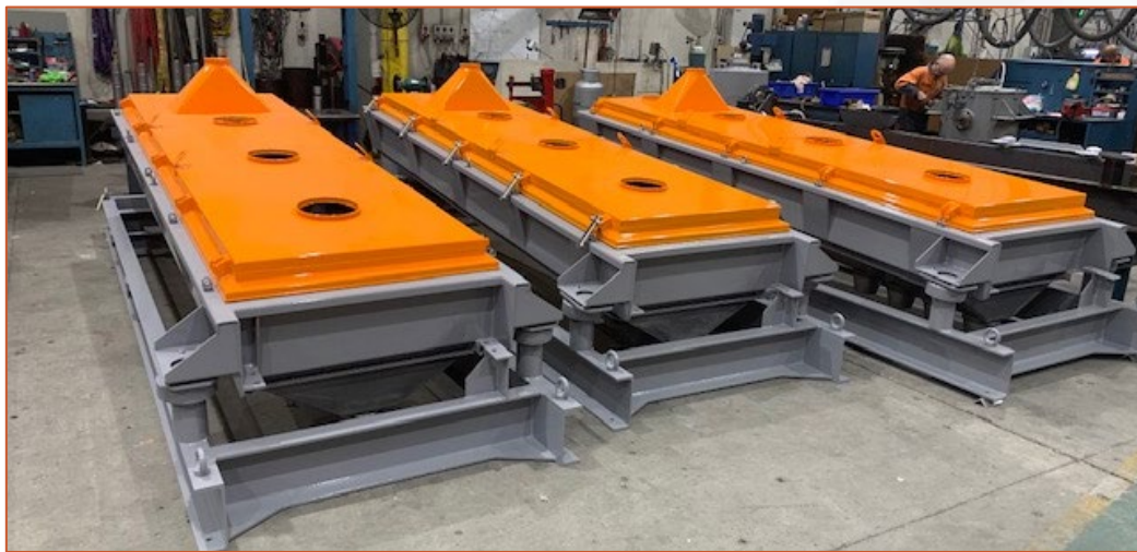
Figure 4: Rotex Screens assembled at the workshop in Melbourne.
