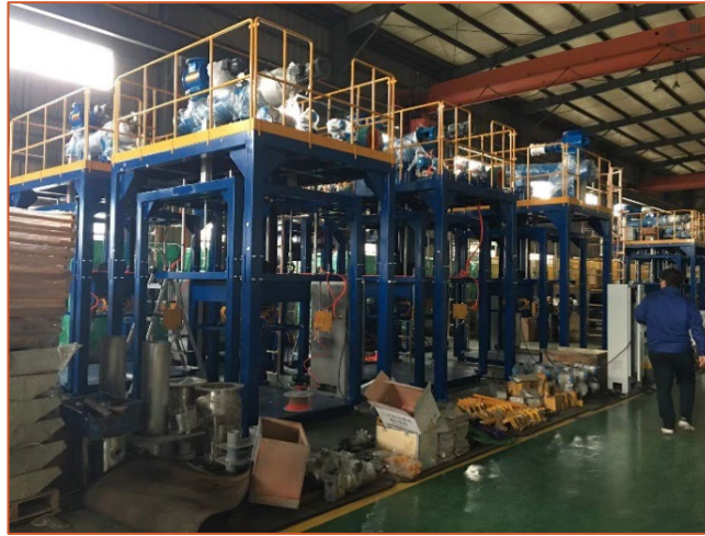
Figure 3: Graphite concentrate bagging equipment undergoing factory testing in China.
