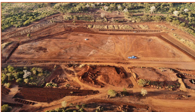
Figure 1: Oblique view from the south of the TSF. Clay filled cut-off keys around the TSF footprint are clearly visible (left). Excavation of the stormwater cut off trench at the TSF (right).
