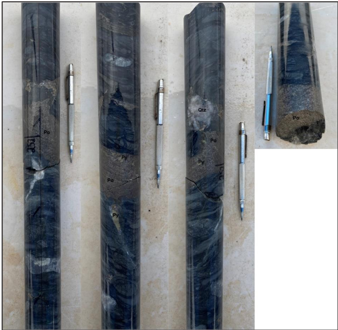
Figure 3: Photo of quartz-pyrite and massive pyrrhotite-pyrite veining within the sulphide alteration zone in KGD003A drill core
