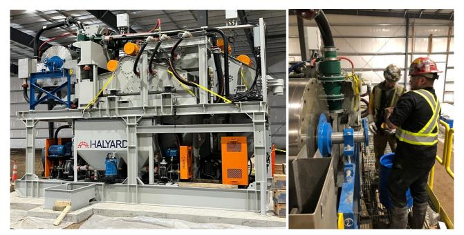
Figures 1 & 2: Commissioning begins for a dense media separation plant at Vital's Saskatoon rare earths extraction facility
