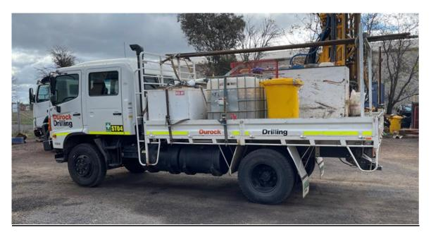
Figure 3: Support Truck, 2,000L of diesel and 1,000L water
