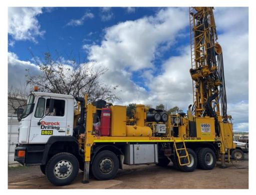
Figure 1: Durock UDR 1000- with a 1150CFM /350psi compressor on board
