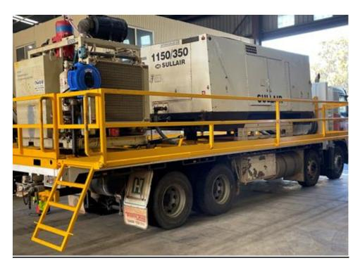
Figure 2: Air truck with 1150CFM /350psi compressor (front) and a 2000CFM/1000psi booster (rear)
