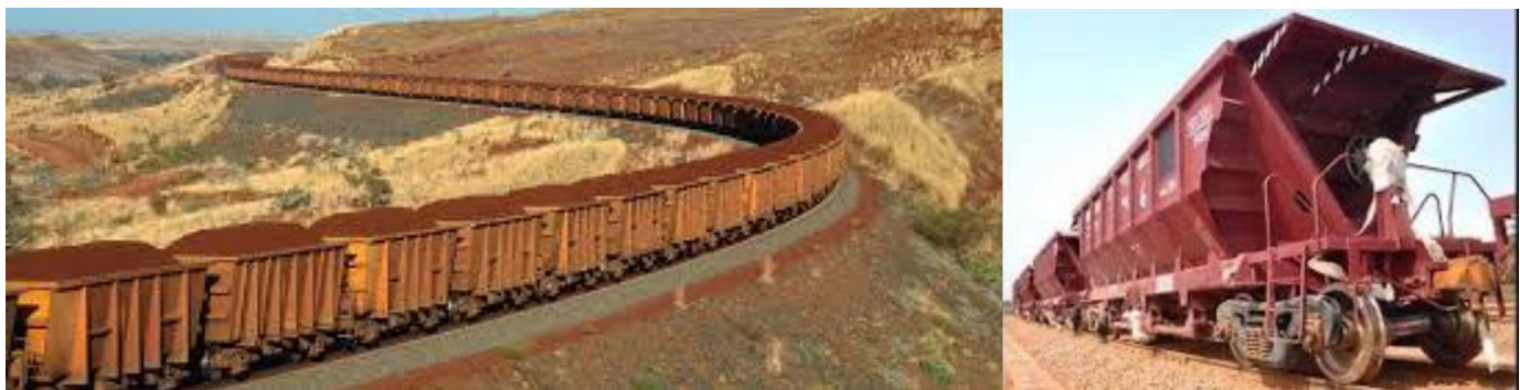
Figure 17: Bauxite ore train and an example of a bottom dump ore wagon
