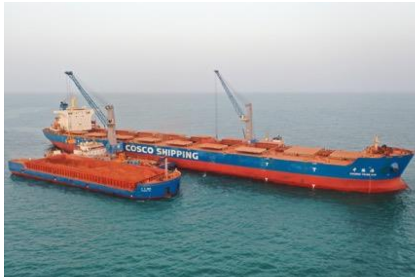
Figure 22: Bauxite being loaded onto a ship with floating crane
