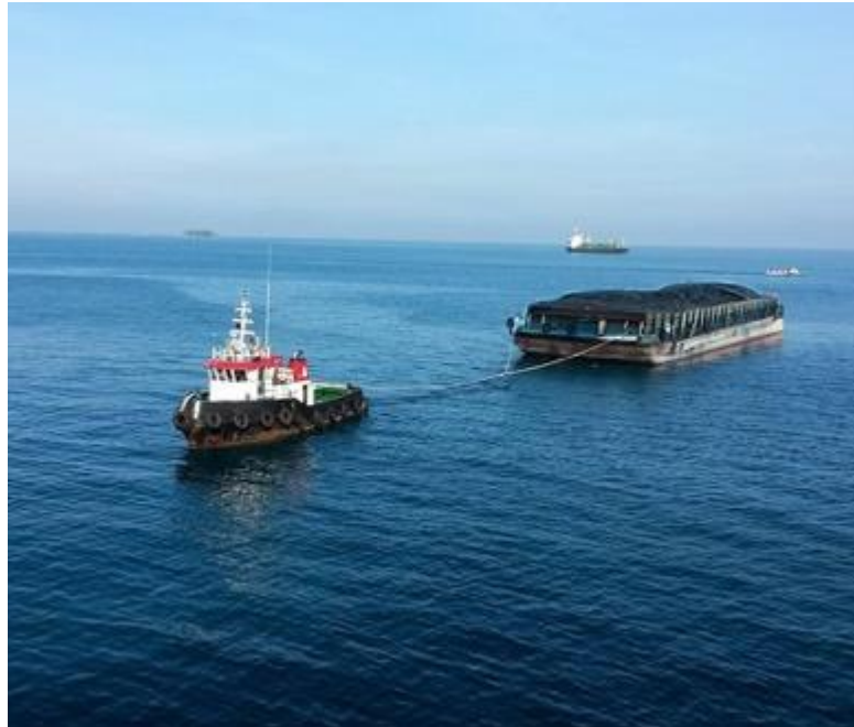
Figure 21: Tugboat towing an ore transshipment barge
