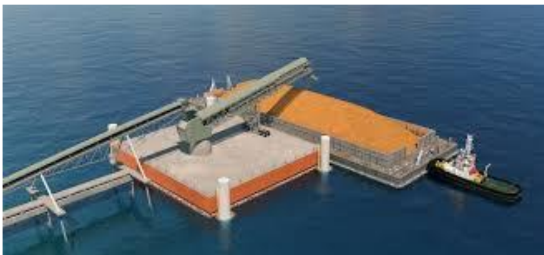
Figure 20: Typical radial telescopic barge loader
