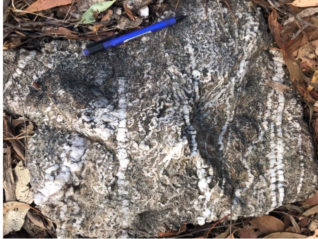
Photograph 2: Missing Link Monzogranite surface outcrop showing intense UST textures (“brain rock”) with overprinting mineralised sheet quartz veins.
