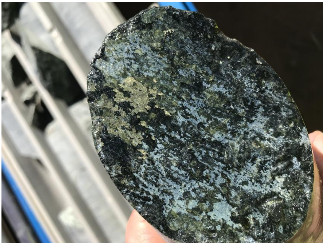
Figure 11 - Diamond Hole - NRDD004 – Nickel and Copper in sulphide at 544.0m
