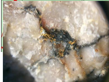
NQ drill core, 47.6mm diameter
