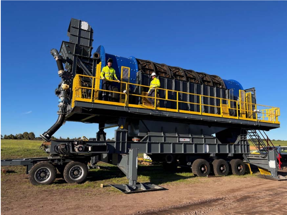
Figure 3 Mobile Mining Unit Plant Trommel
