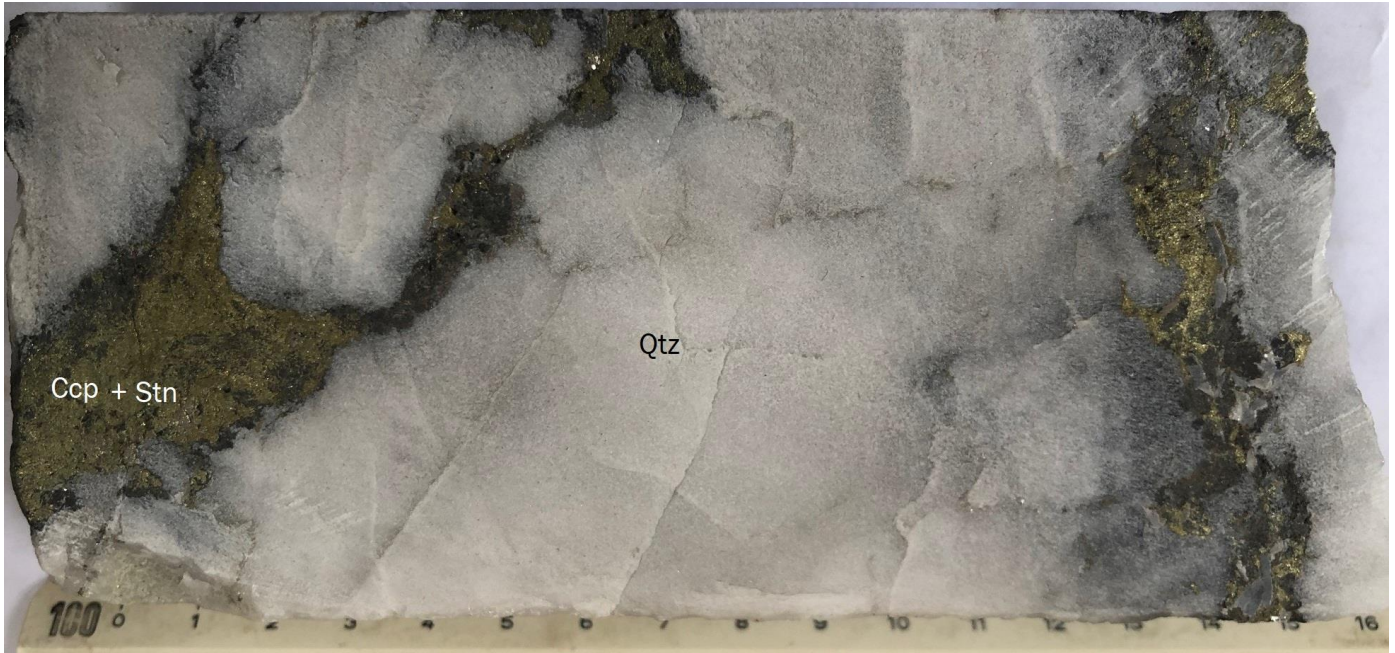
Figure 8. Milky quartz vein including irregular clusters of chalcopyrite and minor stannite of centimetric size randomly distributed within the vein. The photo is from ddh PN01, at a depth of 296.40m. This corresponds to sample 2200128, from 295.70 to 296.80m (1.10m), for which, assay data from ALS returned 0.59% Cu and 0.21% Sn. Previous reported visual estimation of geologists has been of 0.5% Cu and 0.5% Sn.
