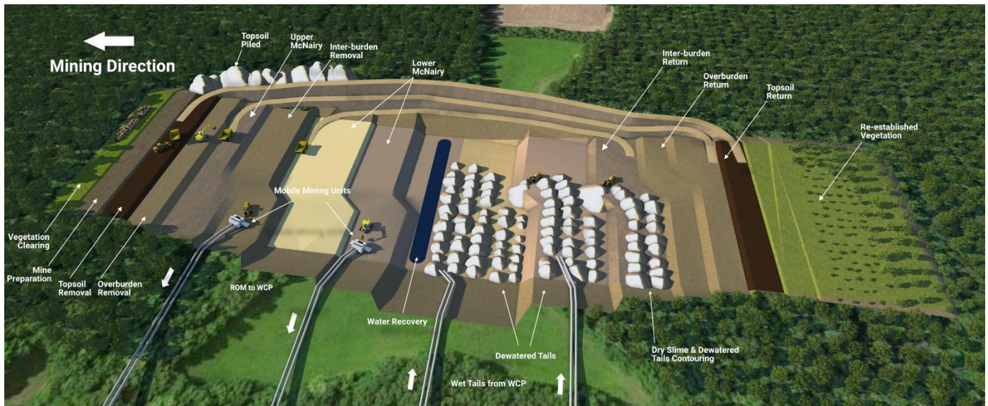
Figure 13: Titan Project mining cycle.
