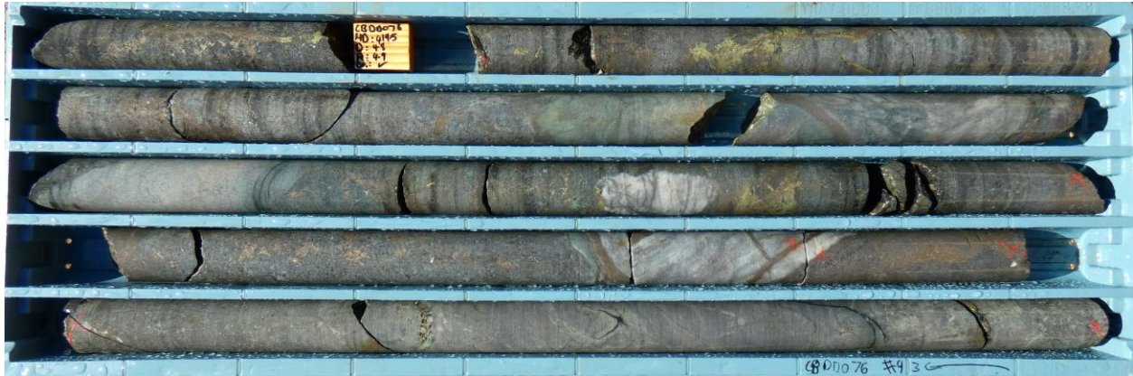
Figure 3: Nickel-copper mineralisation in CBDD076 at 415m downhole, within the sulphide-silica plume. The silica is as a result of the intrusion exhuming sulphur-rich country rock which then melts and releases sulphur.
