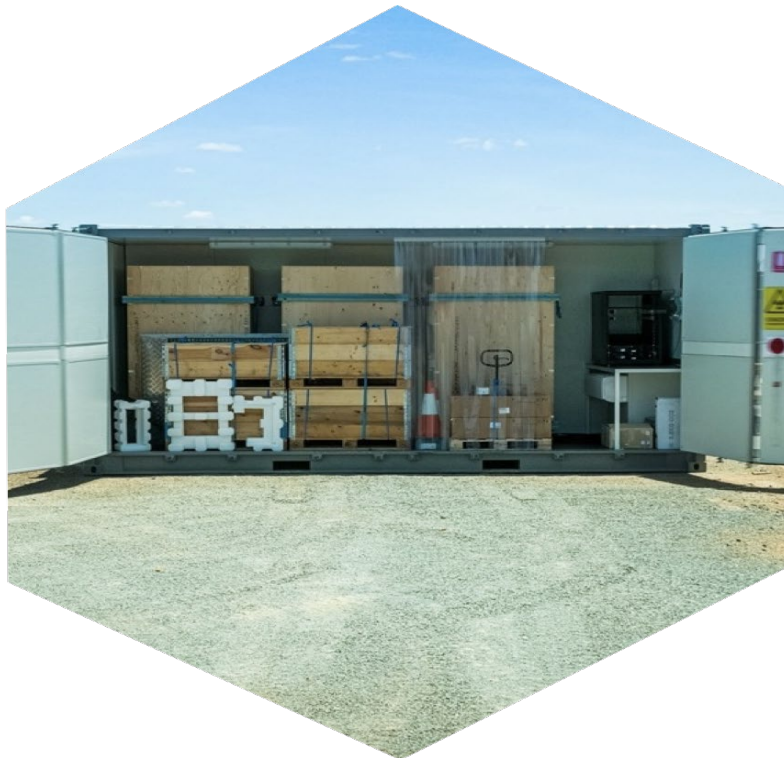
Figure 1: Orexplore self-sustained containerised unit with 3 x GeoCore X10® units
