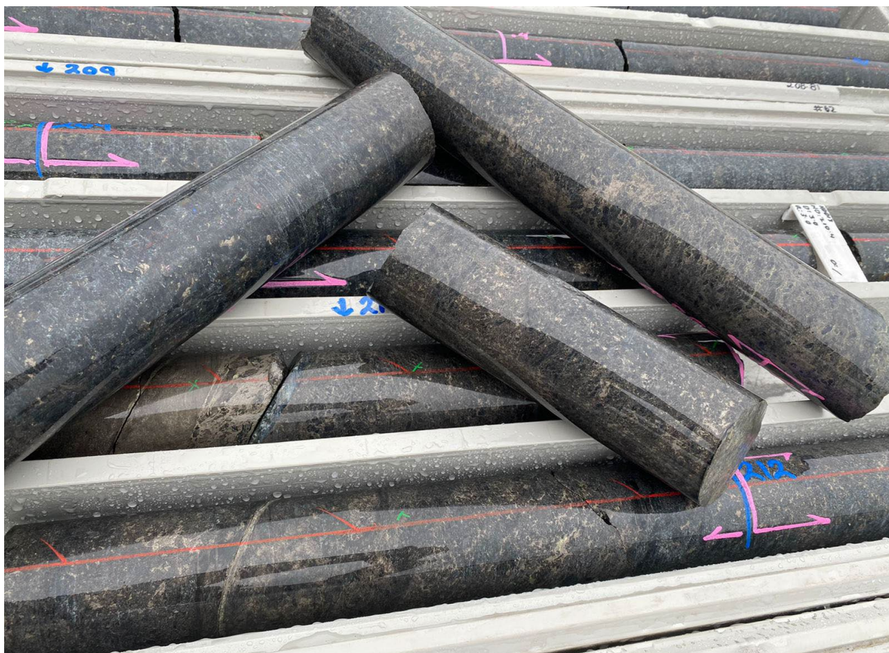
Figure 1. HD013 core specimen photos from matrix sulphide zone (208.6-212.4m).
