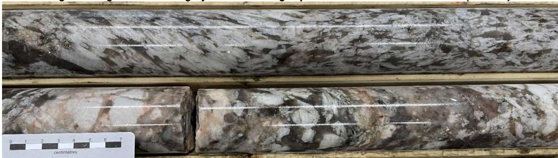
Figure 1: Significant white-grey medium to large spodumene laths within MF22-95 (Hole 36)
