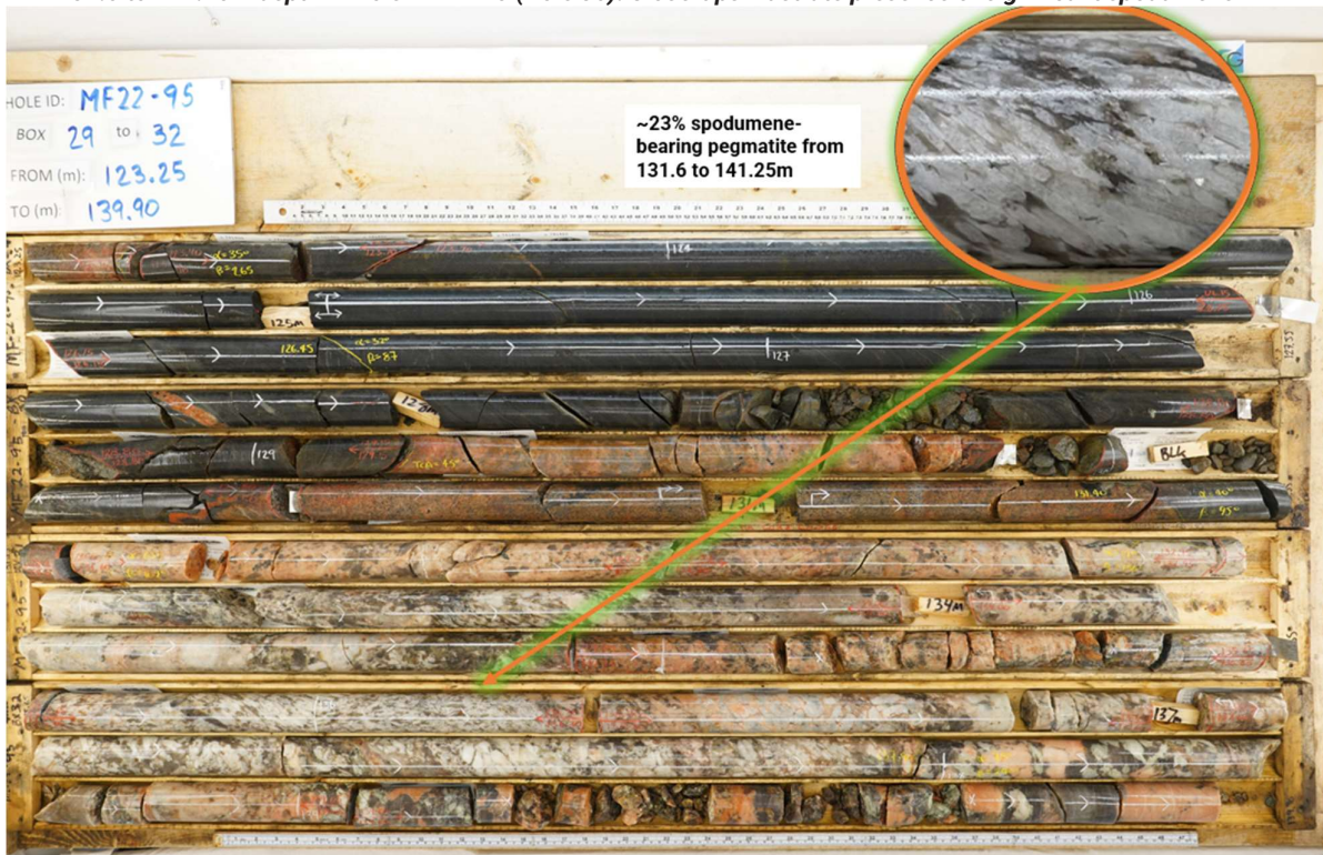
Figure 3: White pegmatite hosts approximately 23% of fine to large, white-grey, spodumene laths intersected from 131.6 to 141.25m depth in Hole MF22-95 (Hole 36). Close-ups illustrate presence of significant spodumene
