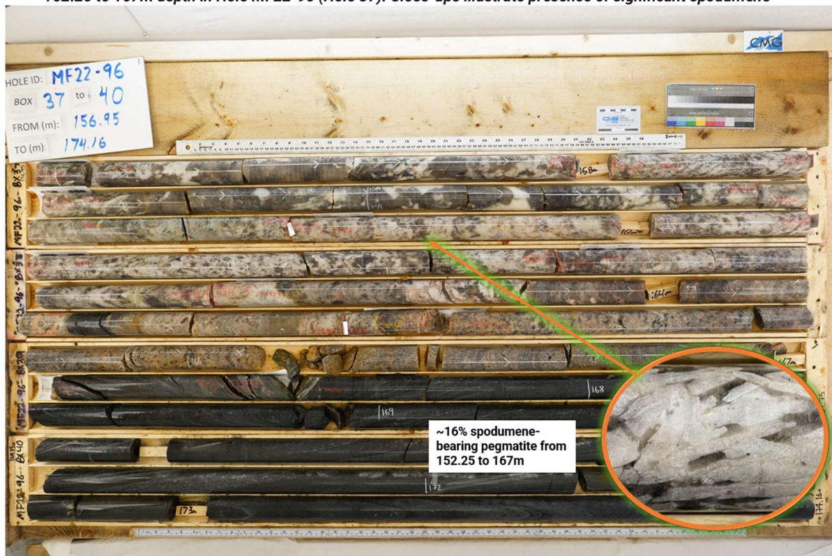
Figure 2: White pegmatite hosts approximately 16% of fine to large, white-grey, spodumene laths intersected from 152.25 to 167m depth in Hole MF22-96 (Hole 37). Close-ups illustrate presence of significant spodumene
