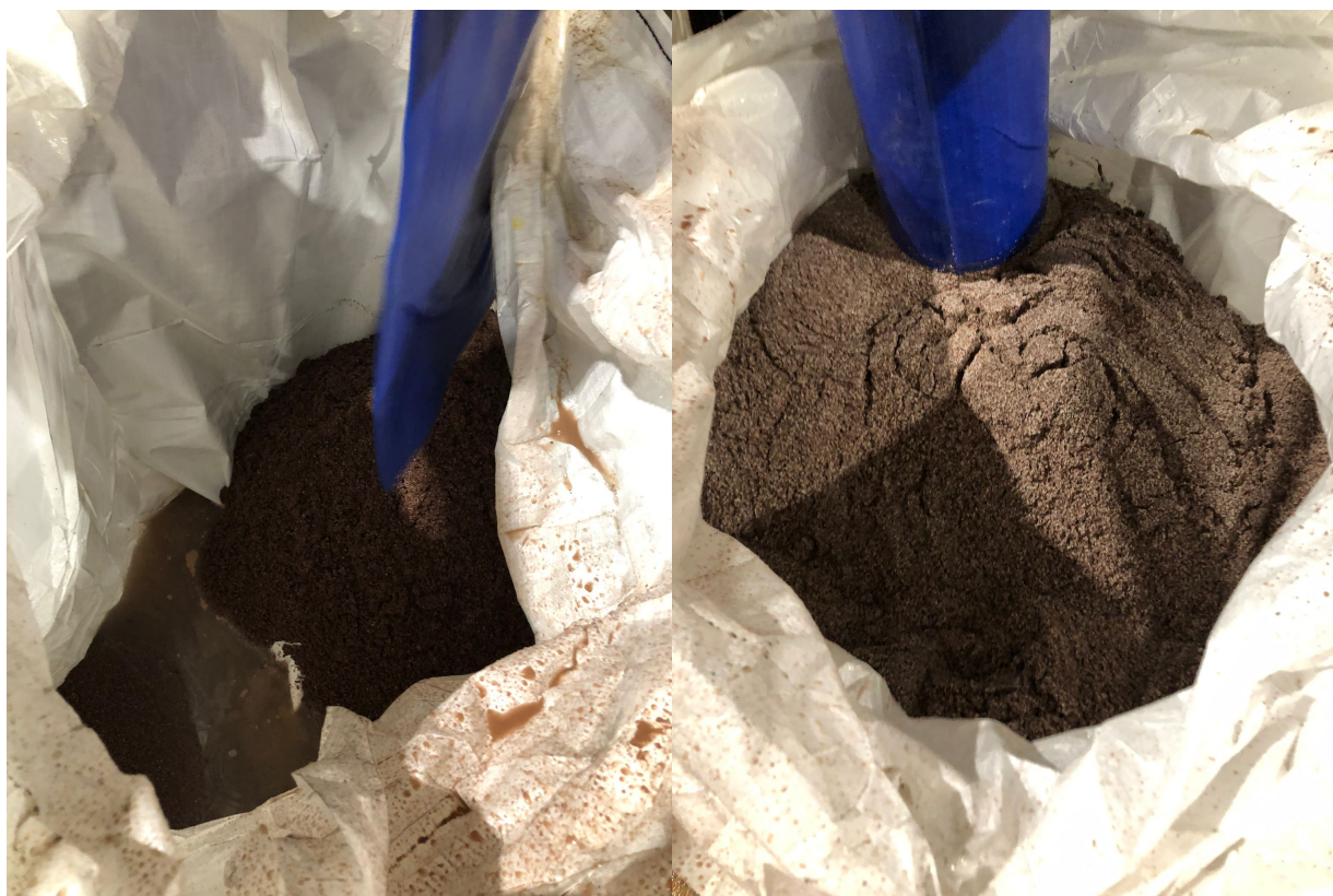
Figures 2 & 3: Concentrate (left) and tails (right) produced during initial DMS commissioning run
