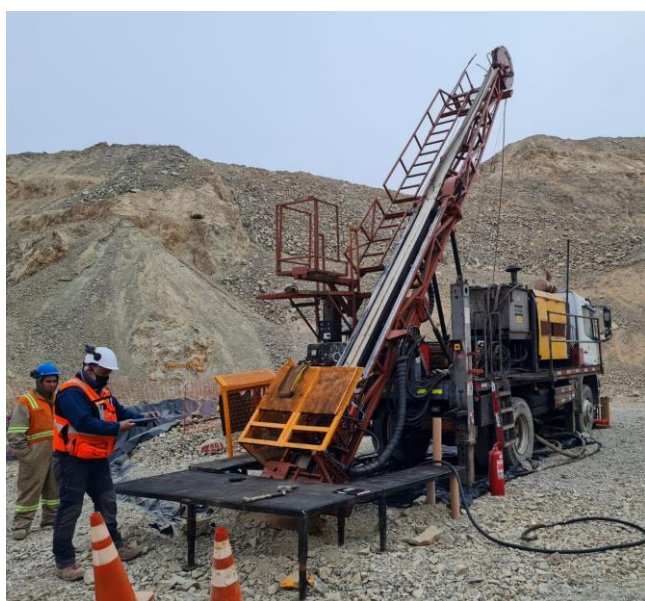
Figure 1 – Diamond drill rigs drilling on ZDDH0297 (LHS) and ZDDH0298 (RHS) at Ternera
