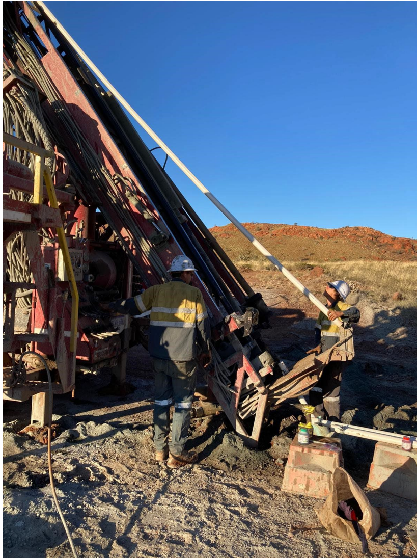
Photo Plate 2: Drilling operation showing drilling team placing PVC casing down the Krona hole in preparation for DHEM Survey.
