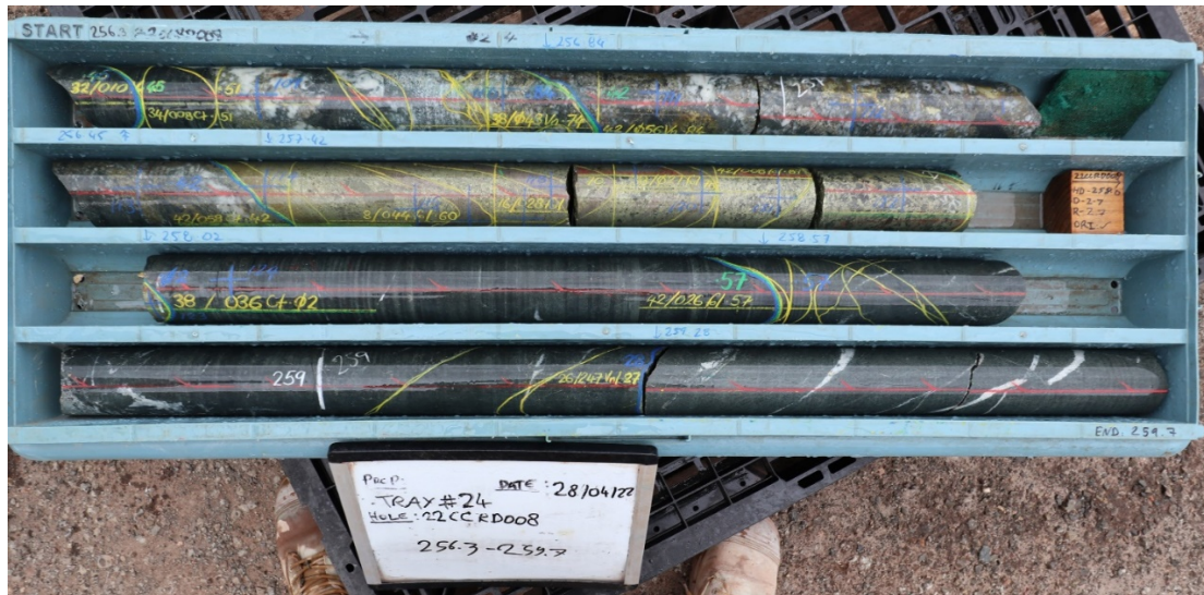
Figure 5: HQ drill core - Part of the upper zone of the broader 16.6m interval showing the massive sulphide zone with brecciated upper contact which returned a result of 1.18m @ 15.65% Cu, 5.40g/t Au, 0.090% Co from 256.84m. Core tray is 1065mm long.
