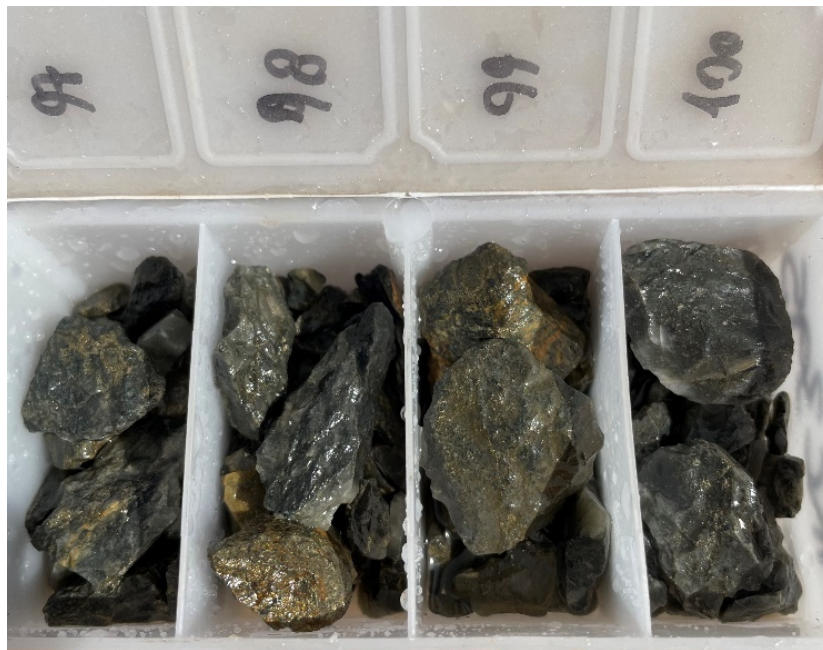
Figure 10: RC drill chips - Sulphide occurrence in Hole ARC395. Assay results are pending for this hole. Each chip compartment is 25mm wide.
