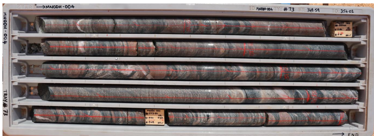
Figure 7: Mulgabbie North Demag Zone diamond drill core MNOBH 004- sericite- carbonate-chlorite altered andesitic volcanoclastic conglomerate with hematite dusting.
