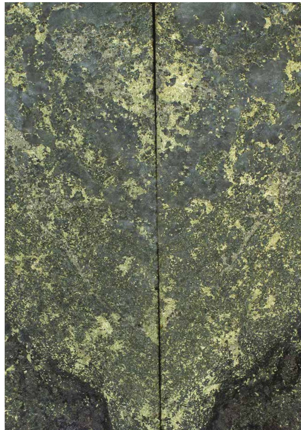
Figure 9. Drill core showing high grade chalcopyrite and pyrite in a late quartz vein.
