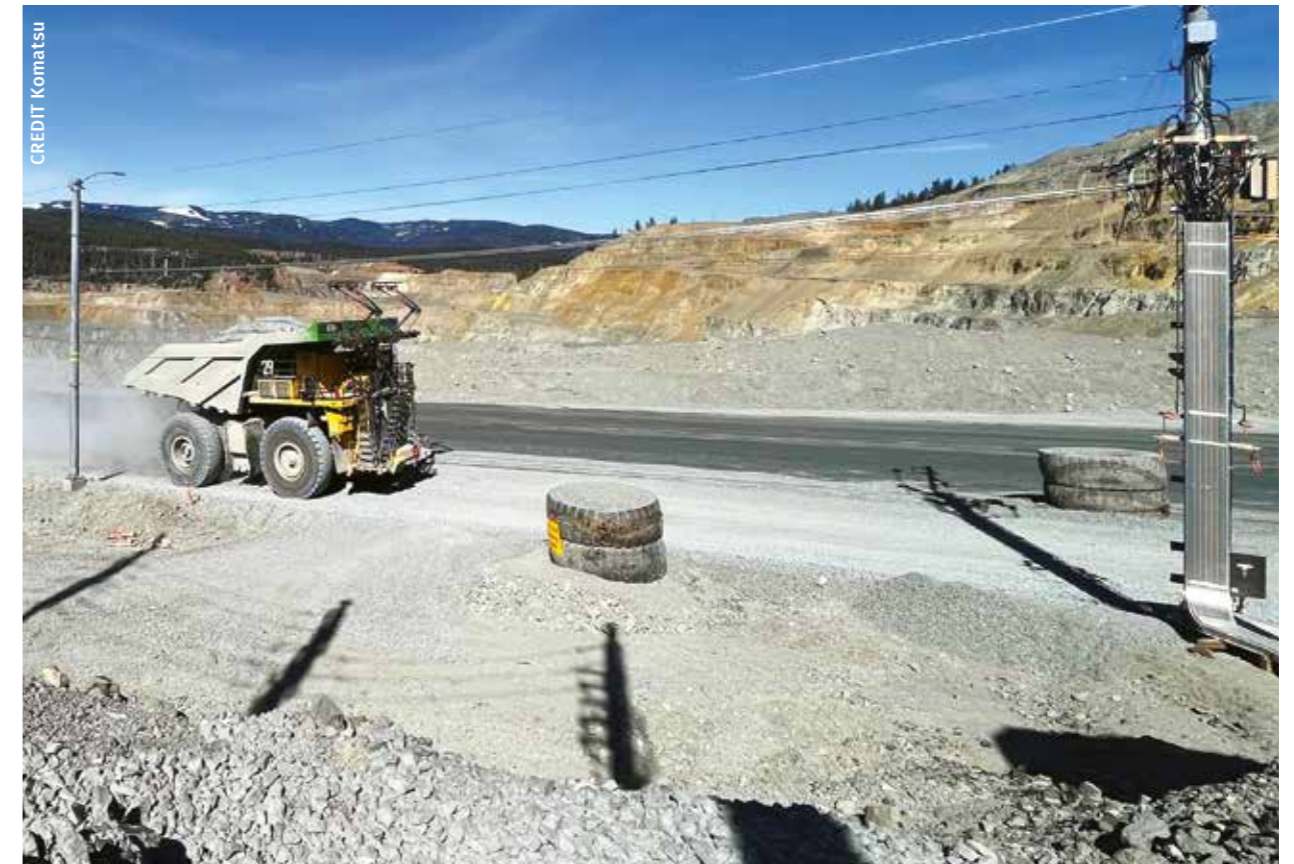
Figure 28: Haul truck with trolley assist at an operating copper production project in Canada.
