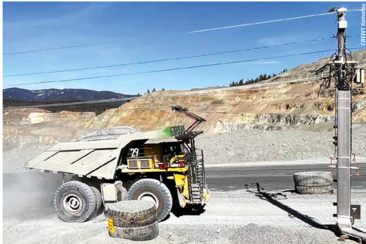
Figure 40: Autonomous mining vehicle on dedicated haul road.
