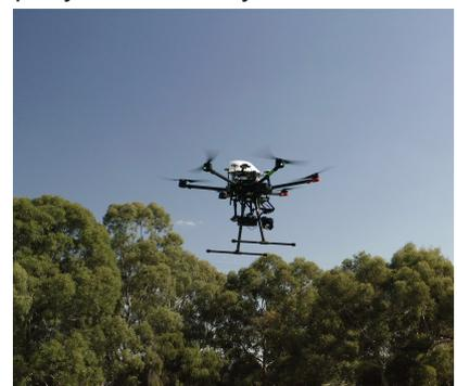
Complete with onboard satellite terminal and all associated hardware at less than 15kg weight, the UAV was locally controlled with no additional hardware or connectivity required at ground control station. This represents a significant opportunity in the global UAV market which is estimated
