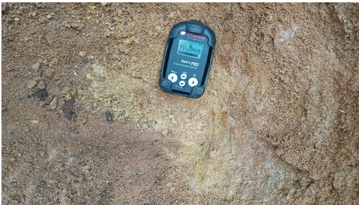
Figure 1. Secondary uranium exposed at surface at Mtonya, the scintillometer reading 40,900 counts per second (40.9 kcps).
