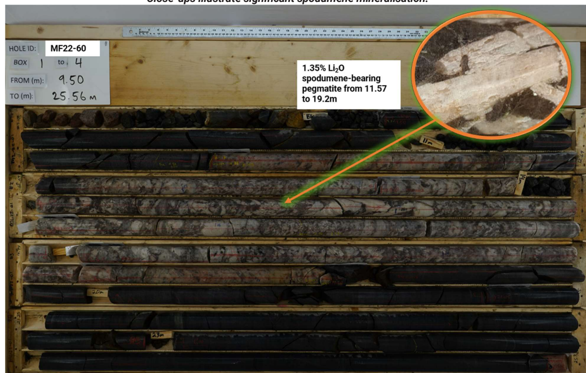
Figure 1: White pegmatite hosts spodumene laths intersected from 11.57 to 19.2m depth in Hole MF22-60 (Hole 01). Close-ups illustrate significant spodumene mineralisation.
