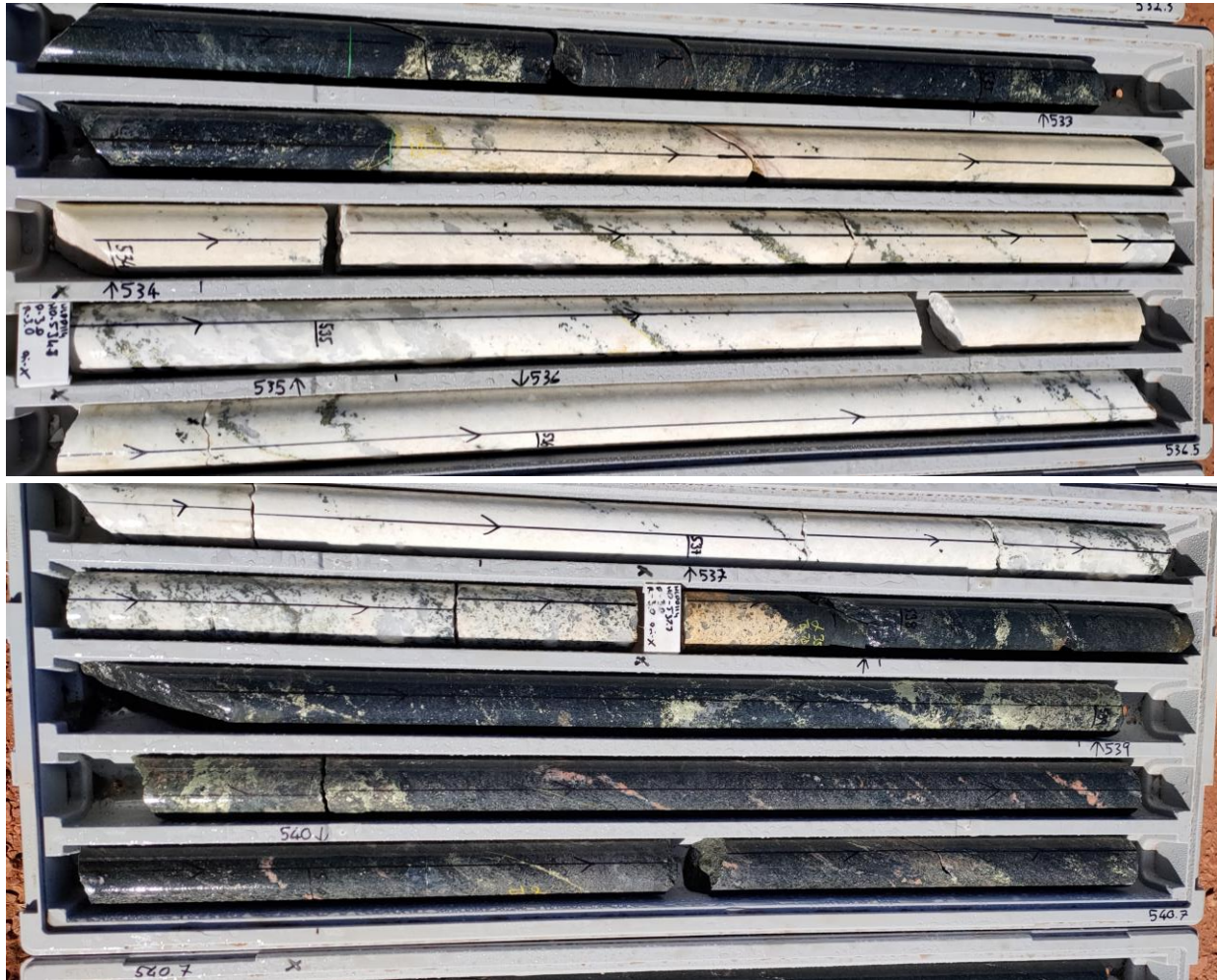
Figure 8. NLDD114 copper sulphide and vein mineralisation.
