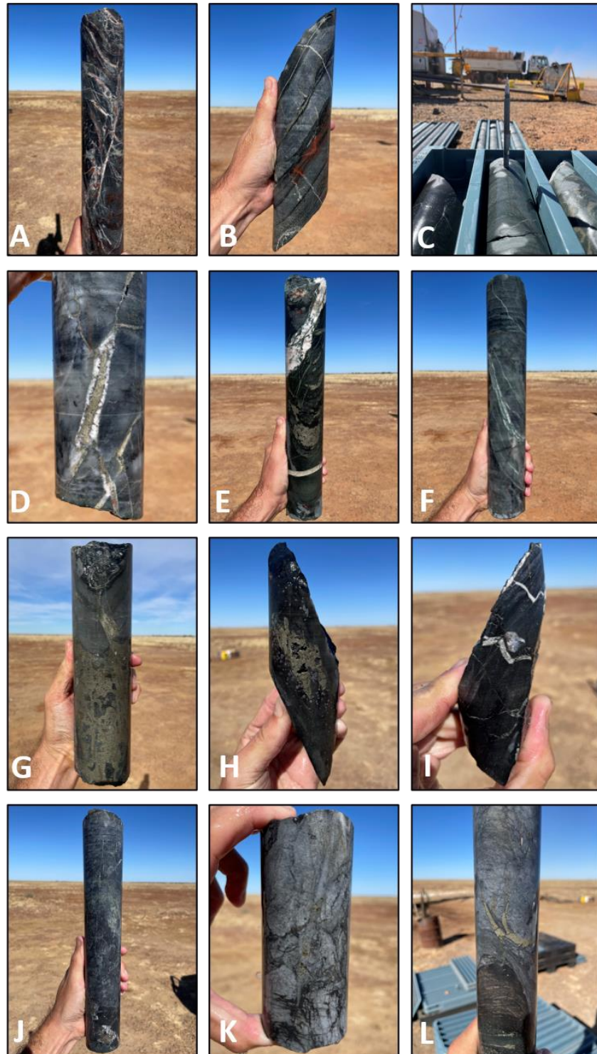
Figure Ap1(A): Core photo collage showing the progression of geology, alteration and veins down FW220009, including: A) haematite-chlorite banded schist with strong quartz-carbonate-haematite veining with ex-sulphides at 222m, B) shale-siltstone intervals with abundant quartz-chlorite-pyrite veins and carbonate-quartz veins with minor haematite at 317.5m, C) magnetite bands in siltstone commence at 319m, D) silicified zone with broken quartz-carbonate veins with disseminated trace-minor pyrite, trace chalcopyrite and low levels of magnetite at 325m, E) strongly chlorite altered shale with quartz-carbonate-chlorite veining, abundant pyrite, and minor haematite and magnetite at 331m, F) silicified zone with abundant chlorite, minor pyrite and haematite, and trace chalcopyrite at 338m, G) strong pyrite-quartz zone within black shale at 367m, H) siltstone-shale with abundant garnet and ex-garnet, strong pyrite-pyrrhotite, and strong chlorite alteration at 407.5m, I) dolomitic veined shale with abundant pyrite and rare sphalerite at 458m, J) dolomitic siltstone with abundant pyrrhotite that becomes increasingly dolomitic and fractured/brecciated with occasional zones of coarser grained pyrrhotite-pyrite-(chalcopyrite) at 480m, K) silicified, brecciated siltstone with dolomite veins, black fracture infill with variable trace-minor pyrrhotite-pyrite and trace chalcopyrite disseminations at 491m, and L) brecciated, silicified dolomite-chlorite veins with pyrrhotite-pyrite with trace chalcopyrite at 508m.
