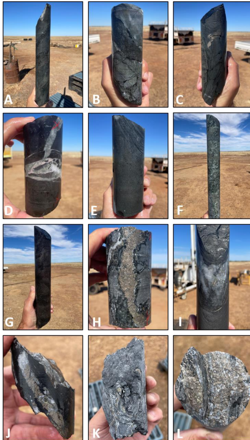
Figure Ap1(B): Core photo collage showing the progression of geology, mineralisation, alteration and veining down the hole, including A) strongly magnetite-rich siltstone hosting variable garnet, pyrrhotite, pyrite, and chalcopyrite at 595m, B) magnetite-rich and silicified, brecciated siltstone hosting minor pyrrhotite with lesser pyrite and trace chalcopyrite at 607.5m, C) magnetite-rich siltstone with pyrrhotite-(chalcopyrite) at 609m, D) narrow vein-breccia zones hosting quartz-epidote-fluorite-chalcopyrite-kspar at 647m, E) magnetite-dolomite siltstone with strong pyrrhotite-pyrite-(chalcopyrite) at 701.5m, F) strong dolomitic alteration overprinting brecciated siltstone at 719m, G) 2.5m wide, semi-massive pyrrhotite-pyrite zone with trace chalcopyrite occurring within a c. 40m wide, intense dolomitic altered zone at 730m, H) pyrrhotite-pyrite-(chalcopyrite) veining within dolomitic siltstone at 795.5m, I) 5cm wide quartz vein hosting pyrrhotite and chalcopyrite in graphitic schist 809m, J) quartz-pyrrhotite-pyrite-(chalcopyrite) veining in broken graphitic schist at 906.5m, K) folded and broken graphitic schist with quartz-pyrrhotite-chalcopyrite at 970.5m, and L) pyrrhotite-quartz-(chalcopyrite) vein on core fracture face at 976.75m.
